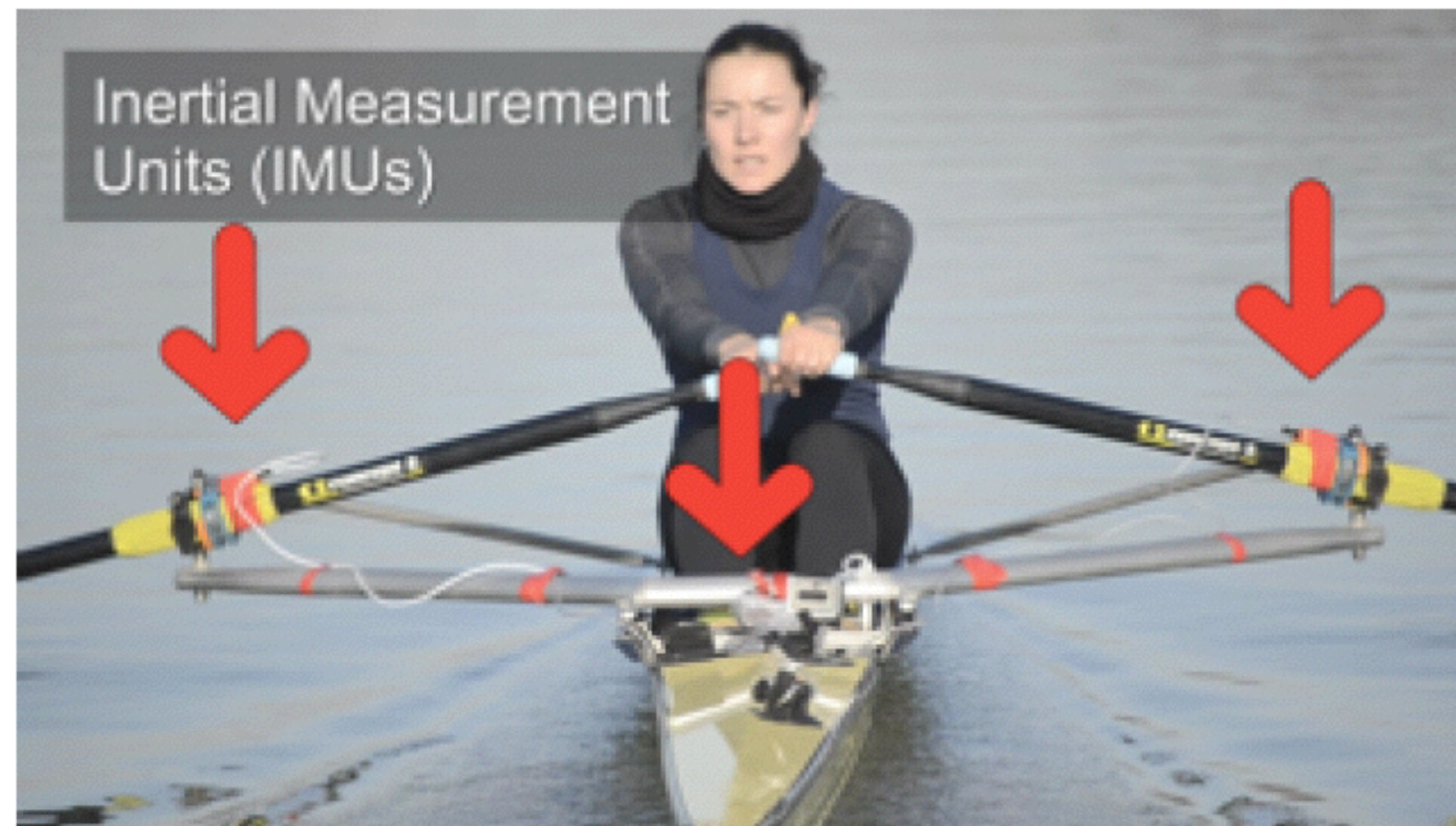
Fig. 5. Implementation of the sensor network: Three IMUs on the oars and the boat, indicated by red arrows.
