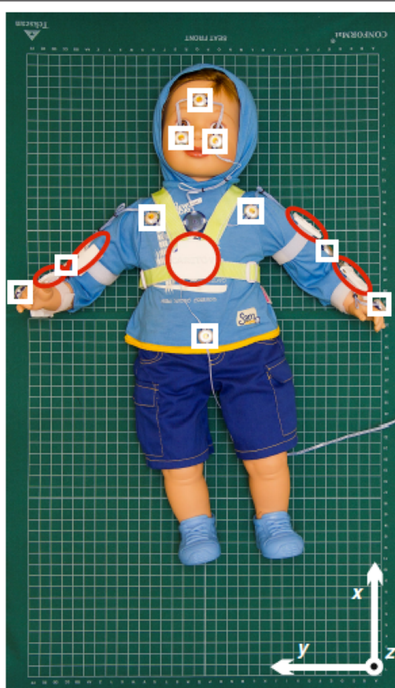
Figure 1 Experimental setup. Baby doll is positioned on top of two pressure mattresses, and equipped with five IMU bracelets (red ellipses), positioned one on baby doll's chest, one on each forearm, and one on each upper arm. Ten Optotrak markers (one on baby doll's forehead, one on each cheek, one on the frontal side of lower abdomen, one on the frontal side of each shoulder joint, one on the lateral side of each elbow joint, one on the dorsal side of each hand) serve as reference (white rectangles). Referential Optotrak and IMU coordinate system orientation is indicated in the lower right corner (white arrows).
